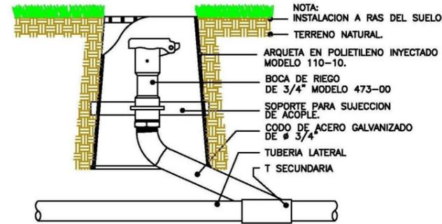
DETALLE DE INSTALACION DE VALVULA ACOPLAMIENTO RAPIDO Ø3/4"
