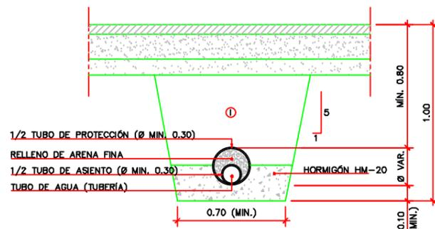
① NOTA: RELLENO DE ZANJAS CON MATERIAL CRIBADO SIN PIEDRAS SUPERIORES A 8 CM. COMPACTADO AL 95% P.M.
