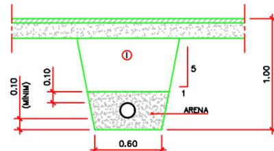
① NOTA: RELLENO DE LAS ZANJAS CON MATERIAL CRIBADO SIN PIEDRAS SUPERIORES A 8 CM. COMPACTADO AL 95% P.M.
